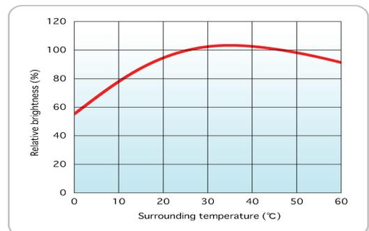
Figure 4. Relationship between relative brightness and ambient temperature
